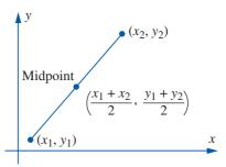
When using coordinate geometry formulae, always allocate one point to be  $(x_1, y_1)$  and the other to be  $(x_2, y_2)$  before you use the formula.
