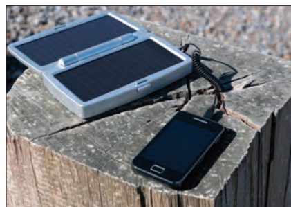
Fig. 16.02.04 A solar-powered battery charger.
